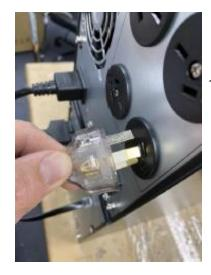
15. Plug your refrigerator into one of the outlets on the back of the UPS.
