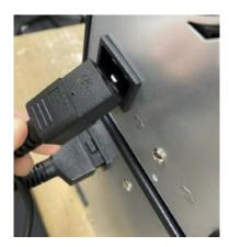
11. Plug in the supplied power cable into the back of the UPS and switch the power on at the wall socket.
