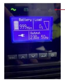
13. The UPS will now come online, and you should have both an input and output value. The output value should be 230v.
