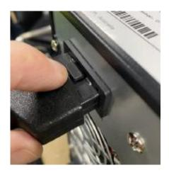
10. If you need to disconnect the battery cable, press down the release and pull out.
