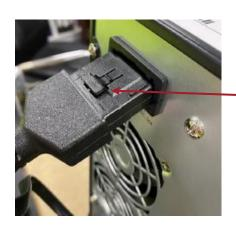
8. Put the cable in the slot at the top of the UPS.
