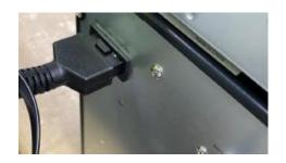
9. Connect the battery cable to the top slot on the battery box.
